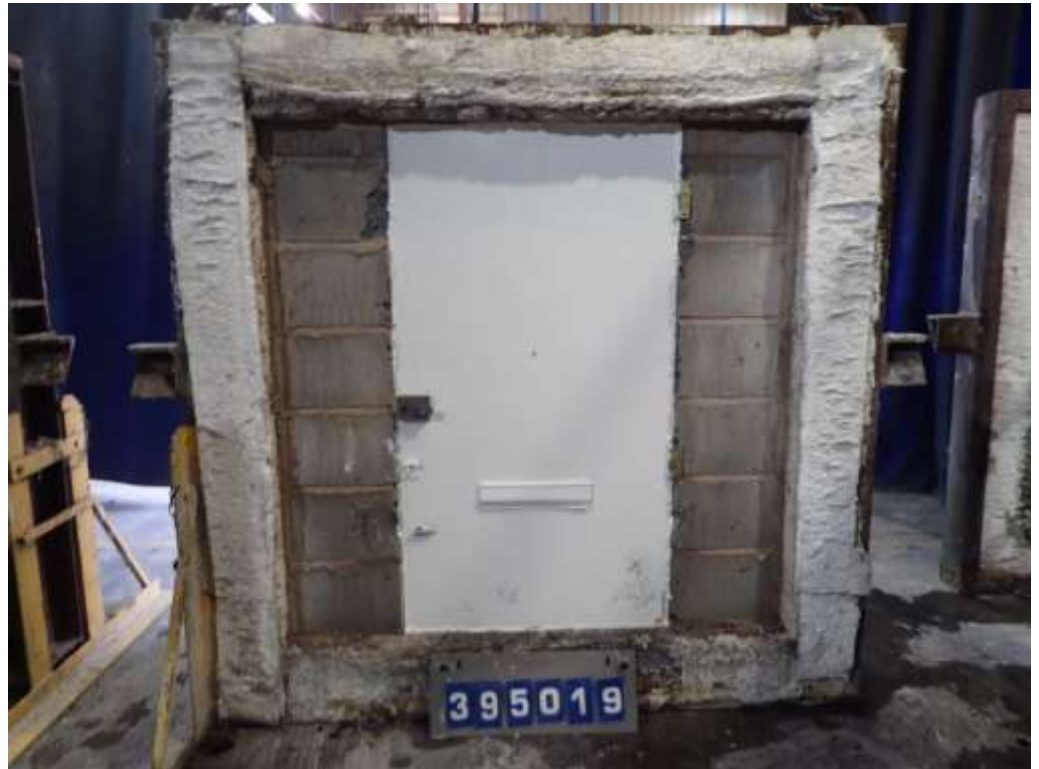
The exposed face of the doorset prior to testing
